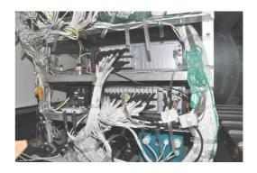
The ability to interchange imc CRONOScompact amplifiers is important for flexible adaption to wide varieties of measurement tasks. The measurement devices are securely installed in the aircraft and the sensors are attached to a customer-specific connector panel equipped with the desired connector types.
