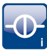
Three-Wire Current Loop 3-wire Sensor with 4 – 20 mA loop current and bipolar Voltage Supply ( \pm 15V )
