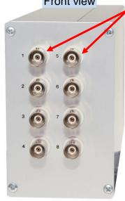
BNC socket for analog signal outputs 1 ... 8
