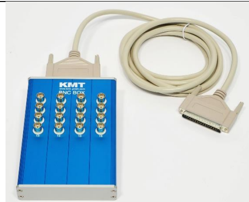
Optional BNC16 Box. Connect on 37pol Sub-D
