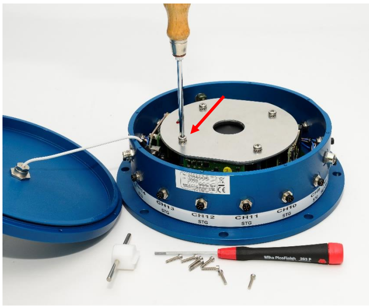
3. Open 4 screws from modules holder ring (screw with spring washer!)
