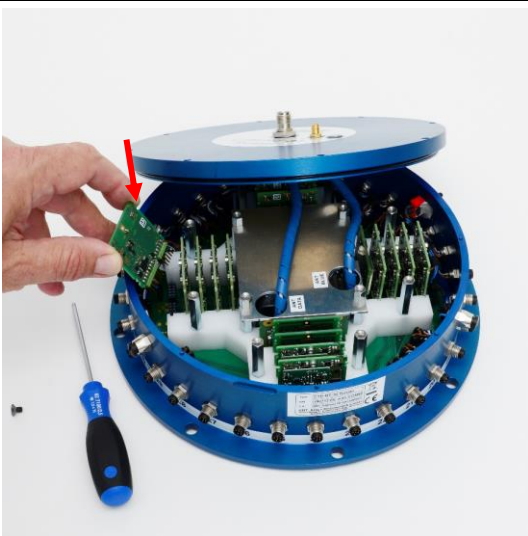
5. Now you can change CTP-NT-Acquisition modules
