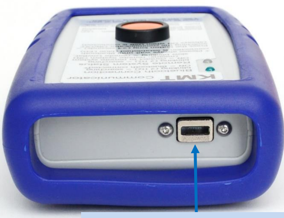
Micro-AB USB Receptacle for powering and communication to PC
