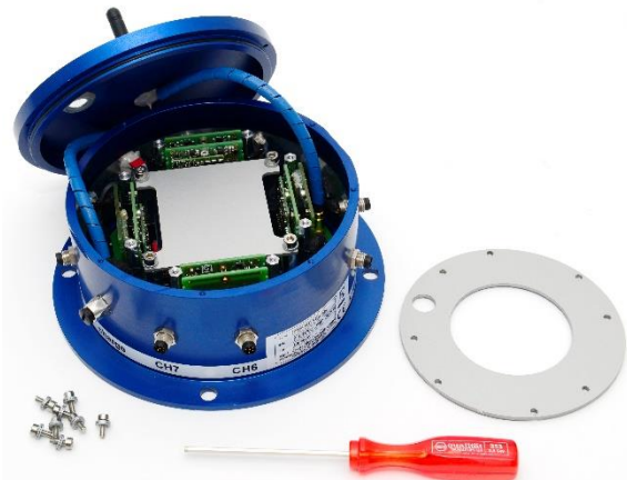
4. Move the modules holder ring to the rear (it is not necessary to disconnect the antenna blue cables)
