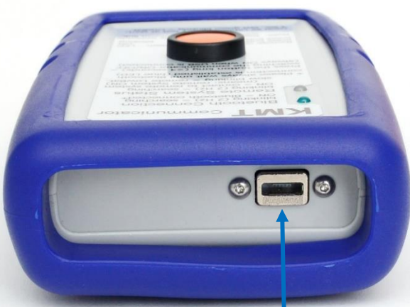
Micro-AB USB Receptacle for powering and communication to PC
