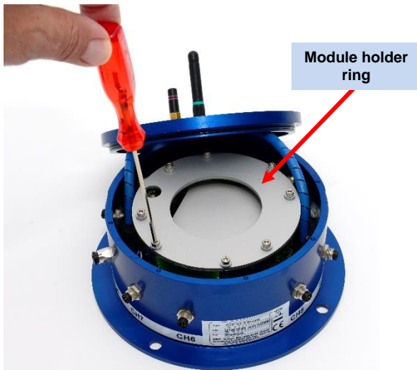
3. Open 8 screws from modules holder ring
