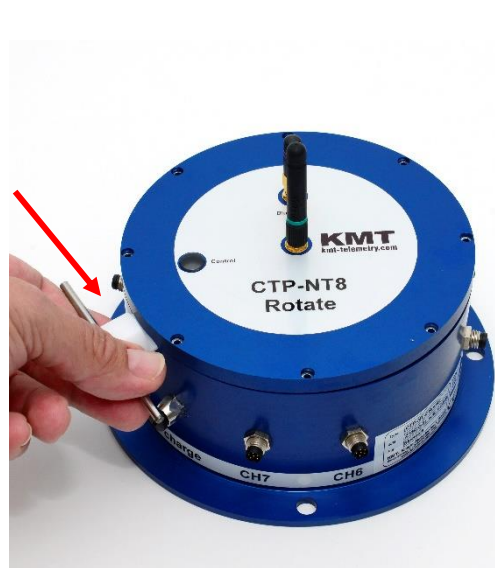
2. Use cover lifter to open the cover carefully
