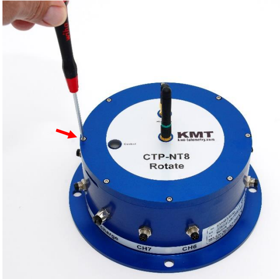
1. Open 8x hexagon screw (2.5mm) with 2mm screwdriver
