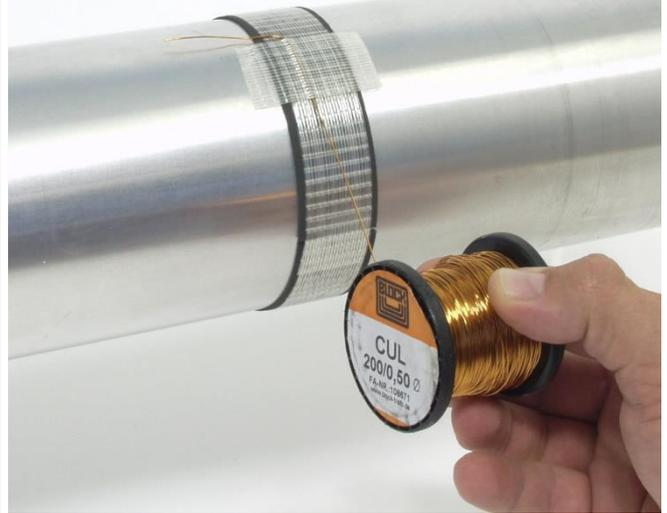
Solder the wires of the coil on the input pins of TEL1-PCM-STG "COIL". The pins for capacitor are used only for larger diameter >400mm!
