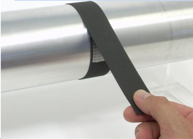
Fix with 2 layers of mounting tape around the shaft
