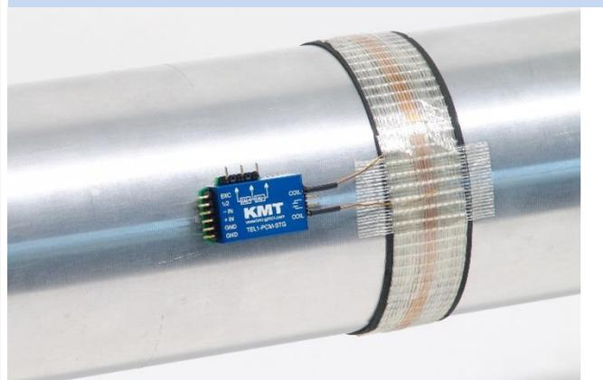
10 layers of the special mounting tape around the shaft. We recommend additionally use of a **hose clamps** for final fixing of the transmitter unit!!
