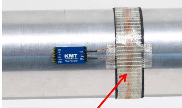
Coil, depends of shaft diameter, 5-18 parallel windings of 0.5 or 0.63mm
